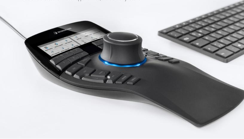
**Professional 3D Navigation in CAD** – Intuitively and precisely navigate digital models or views with the patented Six-Degrees-of-Freedom (6DoF) sensor.
