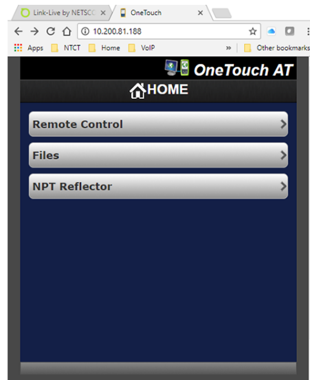
Figure 13: OneTouch web server for remote file retrieval and/or download the NPT Reflector software.
