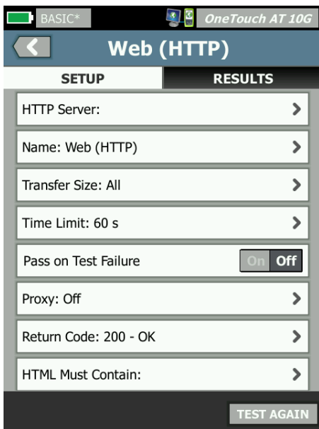
Figure 8: Connectivity and response test against the web server can include verification of respond code and text.
