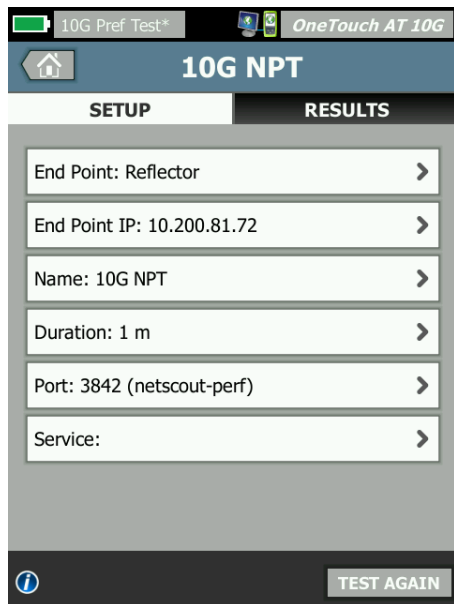
Figure 16: 10G NPT tests up to 10G against reflector, peer or OptiView XG over a user defined UDP port.
