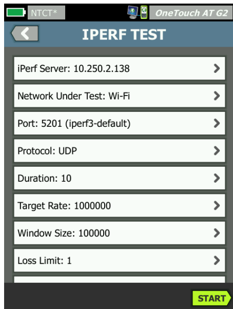
Figure 21: Setup for TCP Window Size and Threshold.
