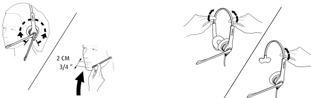
Jabra Biz 1500 has a 270° boom arm so it can be easily adjusted without breaking.
