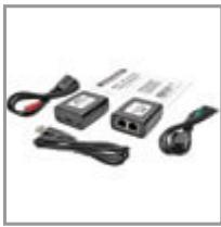
Transmitter and receiver work in tandem to extend HDMI audio/video and IR control signals via Cat5/6 cable to a display up to 100 ft. Ideal for digital signs, schools, retail settings and trade show presentations.
