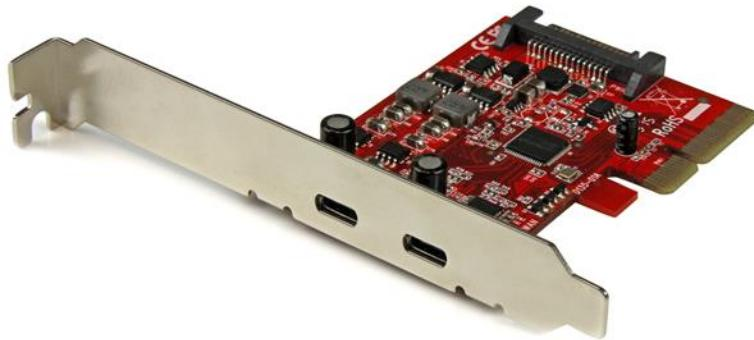
Get ready for the future of universal connectivity and high-speed performance. This USB 3.1 card adds two USB-C™ ports to your desktop, with a combined bandwidth up to 10Gbps. With greater bandwidth, you can save time and avoid the performance bottlenecks often associated with other connectivity technologies.
