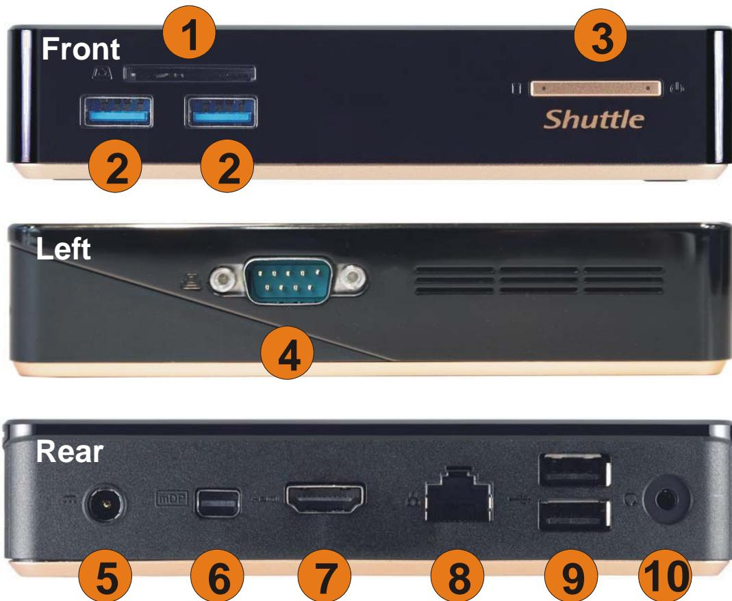
**1** Card reader**2** 2x USB 3.0 (2A charging current)**3** On/Off Button with 2 LEDs**4** RS232 COM port**5** DC input for external power adapter**6** Mini-DisplayPort**7** HDMI**8** Gigabit LAN (RJ45)**9** 2x USB 2.0**10** Audio Combo Port 3.5 mm:
