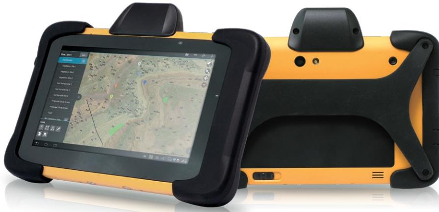
The DT307GS GNSS Tablet features the integration of a brilliant 7" capacitive touch screen and a quad-core, energy efficient processor within a slim, lightweight and durable package. With its high-accuracy GNSS module, Android operating system and optional camera module, this tablet is compatible with existing GIS software for surveying and mapping applications and brings together the advanced workflow for GIS data capture, accurate positioning, and data transmitting.
