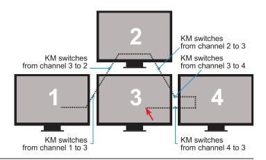
The Belkin Advanced Secure KM Switch makes it possible to use multiple secure systems on separate displays simultaneously with a single mouse and keyboard.
