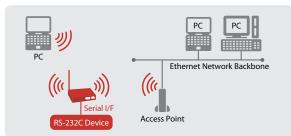
Wireless Access Point Mode: The SD-310AN can create a wireless network so any wireless client (station) can easily make a direct secure connection.
