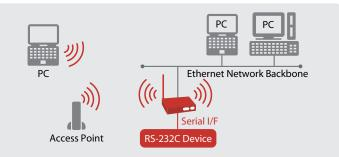
eCable Mode: Serial data can be tunneled over the network between devices connected to SD-300/SD-310AN.
