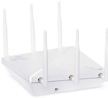
The **AP390** is an enterprise-grade, high performance two radio (3x3) three stream MIMO 802.11ac/n Access Point, targeted at high capacity best range enterprise environments with external antenna and extended temperature option.
