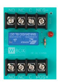
Applications include intrusion, access control, video surveillance and other systems requiring control or activation of electronic devices. Operations include dry contacts, latching dry contacts, polarity reversal and line seizure. Includes double-sided foam mounting tape.
