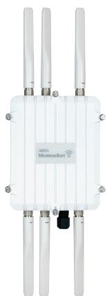
The Bluesocket 2125 APs include six N-type connectors for external antennas, and are fully functional with power delivered by a single port 802.3at (PoE+) solution.
