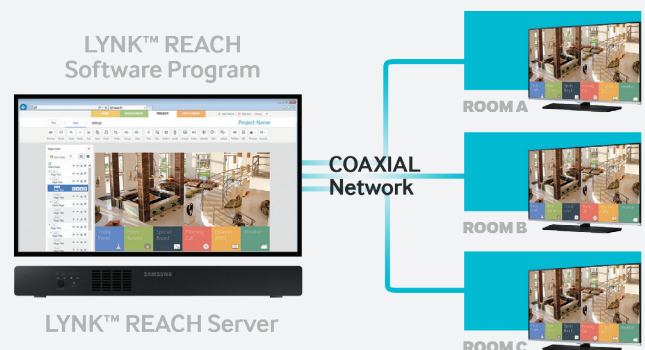
Figure 3. LYNK REACH offers a flexible and low-cost coaxial infrastructure Hospitality TV solution
