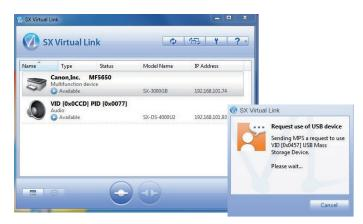
The software discovers USB Device Servers and USB devices on the network, and the search results are shown in an overview on the main screen.
