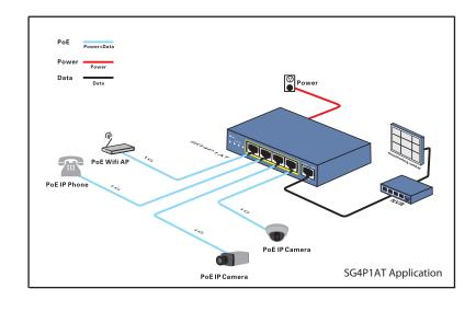
of a PD (Powered Device). The switch will be able to determine if power is to be supplied to any of the PoE supported ports. This helps in the reduction of power used by the switch to power unused ports as well as insuring that power is not put out on wiring that is not connected to a PD.
