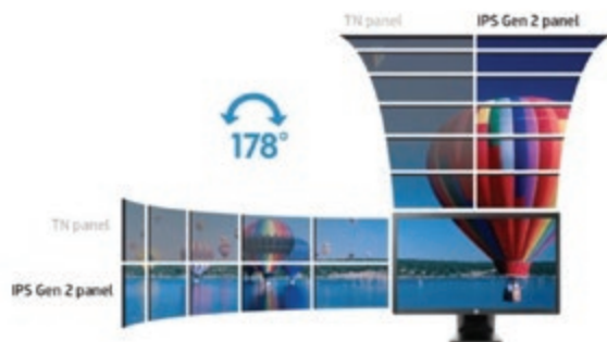
Figure 1. The effect viewing angles have for IPS and TN displays
