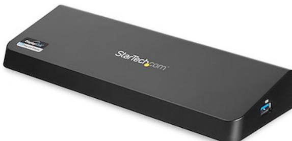
This TAA compliant dual-monitor USB 3.0 docking station combines a 4-port USB 3.0 hub, headphone and microphone audio connectors, a USB fast-charge port, and a GbE RJ45 Port with Wake-on-LAN (WOL).
