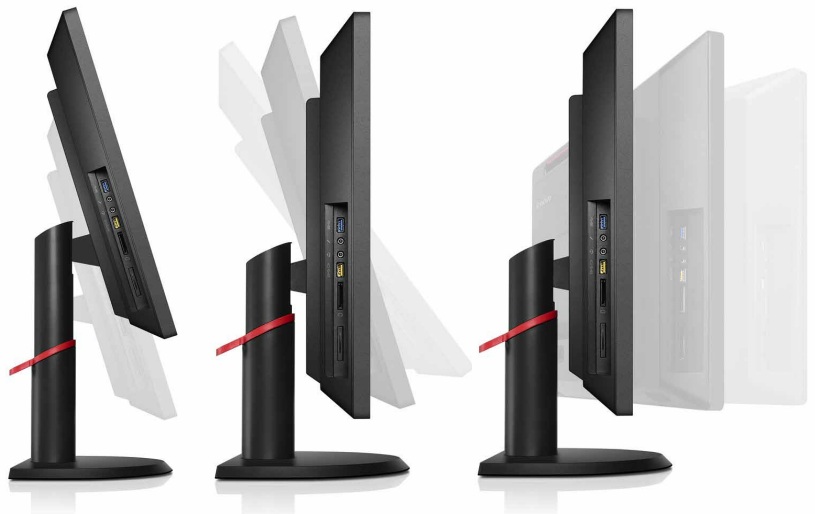
Monitor Stand (Tilt: 45° back, -5° forward; Lift: 110mm; Swivel: +/-45°; Pivot: Landscape / Portrait)
