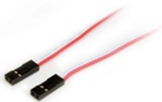
The IDC2PIN12 Motherboard/HDD LED cable features two 2-pin IDC header connectors, enabling you to connect your system LED panel status lights to your motherboard or hard drive controller.
