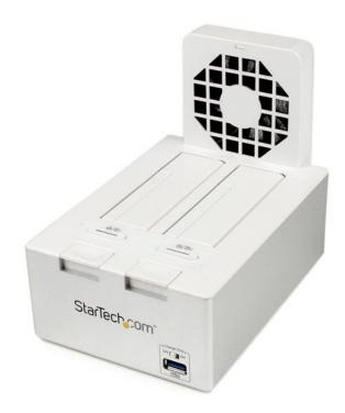
The SDOCK2U33HFW USB 3.0 Dual hard drive dock with Fast Charge USB hub enables two SATA 2.5in or 3.5in hard drives (HDD) or solid state drives (SSD) to be connected simultaneously to a computer through USB, while controlling the power status (on/off) of each individual drive independently from the other. The enclosure supports UASP and delivers optimal performance with a USB 3.0 connection, but is also backward compatible with USB 2.0/1.1 host connections.
