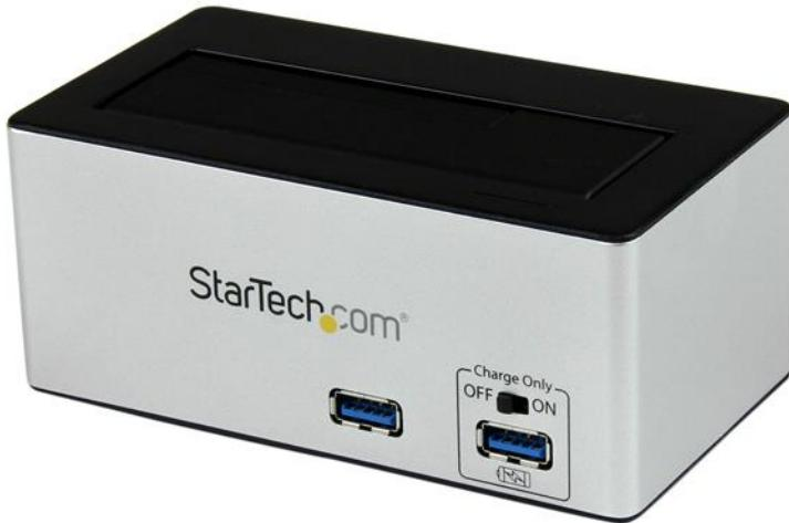
The SDOCKU33HB USB 3.0 hard drive dock with Fast Charge USB hub lets you easily connect and swap 2.5in or 3.5in SATA III hard drives (HDD) and solid state drives (SSD) through an available USB port. The enclosure supports UASP and delivers optimal performance with a USB 3.0 connection, but is also backward compatible with USB 2.0/1.1 host connections.
