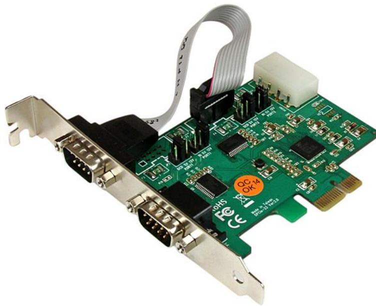
The PEX2S553S 2-Port PCI Express Serial Card lets you add two ESD-Protected RS232 ports with 5V or 12V selectable power output, through a PCI Express slot.
