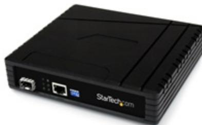
The ET1110PSE PSE/PoE Media Converter, which features an open SFP slot, enables you to create an Ethernet-Fiber link by transparently converting from 1000Base-SX/LX fiber to 10/100/1000Base-T, while acting as a Power Sourcing Equipment (PSE) device.
