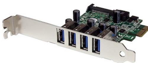
The PEXUSB3S4V PCI Express USB 3.2 Gen 1 Card (with SATA Power) adds 4 external USB 3.2 Gen 1 ports to any PCI Express-enabled computer system with support for data rates up to 5 Gbps, while remaining backward compatible with USB 2.0 / 1.x devices.
