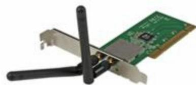
The PCI300WN2X2 Wireless-N PCI Card adds high speed 802.11n network connectivity to almost any PCI-enabled desktop/workstation PC. Using a 2T2R (2 Transmitter/2 Receiver) design over the 2.4GHz frequency, the card supports 300Mbps data bandwidth over an 802.11n network, while providing optimal signal reception and range - the ideal WiFi card for Desktop PCs.
