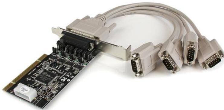
The PCI4S954PW 4-Port PCI Serial Card (with Power Output) turns a PCI slot into 4 RS232 (DB9) serial connections and enables compatible devices to draw power from the serial ports.
