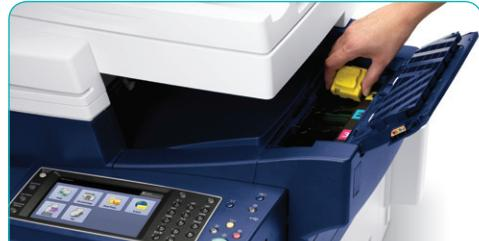
Each Solid Ink stick is uniquely shaped to fit the correct slot, making ink loading fast, easy and clean.
