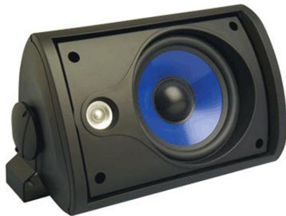
The 3000 Series Outdoor Speakers are optimized for the demands of outdoor installations and come in white or black finishes. With 5.25" poly woofers and PEI mylar tweeters, these speakers are made with tough non-corroding enclosures that feature aluminum powder coated grills and mounting brackets and a universal 1/4-20 threaded insert for accepting 3rd party mounts.
