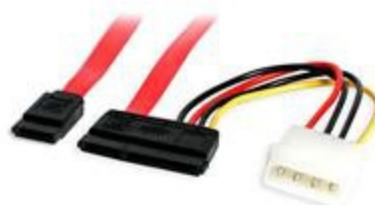
The SATA6POW SATA Data and Power Cable features a combination 22-pin SATA receptacle data and power connector as well as an Molex (LP4) power connector and SATA receptacle data connector, allowing you to create a conventional Serial ATA data connection to a computer while powering the drive through an LP4 connection to the computer power supply.
