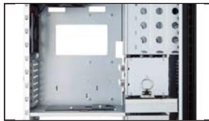
Divided upper and lower chamber structure – the power supply resides in a separate chamber with dedicated cooling from a 120 mm fan to isolate heat from the system and lower system noise
