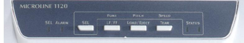
The operator panel of the ML1120 is uncluttered and uncomplicated—which makes it easy to use.
