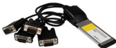
The EC4S952 4-Port ExpressCard-based Serial Card lets you add four RS232 serial ports to your laptop or ExpressCard equipped desktop computer, using an available ExpressCard slot.
