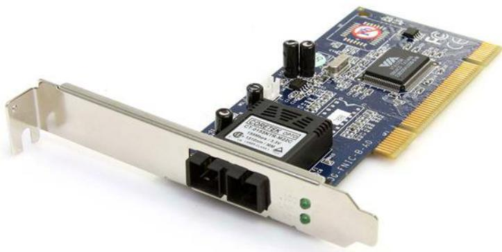
The PCI100MMSC 100 Mbps Fiber Optic (MM SC) PCI Ethernet Adapter Card offers the perfect "Fiber-to-the-desk" solution allowing you to add a multimode SC fiber port to your system through an available standard or low-profile PCI slot.
