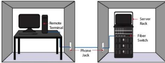
Connect remote workstations to your network over extreme distances using a single secure fiber cable
