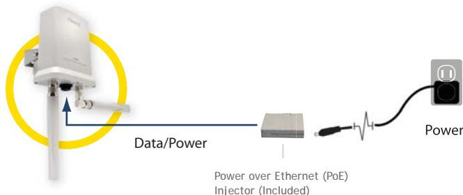
By combining your power and data connections into a single cable, PoE simplifies the setup of the Hi-Gain™ Outdoor Wireless-N Dual Radio Smart Repeater. The included Power over Ethernet DC Injector provides power and network access (through your home or business router or network connection), and combines them into a single RJ-45 connection for the HOW2R1. This allows you to install the HOW2R1 outdoor in hard to reach locations without worrying about running both power and Ethernet cables.
