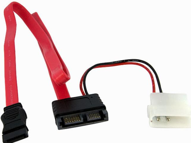
StarTech.com's Slimline SATA to SATA Adapter Cable features one SATA (7-pin) female data connection as well as an LP4 power connection on one end, and a slimline Serial ATA male connection on the other - allowing you to connect a motherboard equipped with a Slimline SATA connector to a standard Serial ATA Drive.
