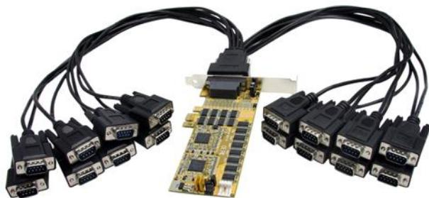
The PEX16S952LP 16 Port Low Profile RS232 PCI Express Serial Card with Cable Included lets you turn a single low profile PCIe slot into 16 RS232 (DB9) serial connections.
