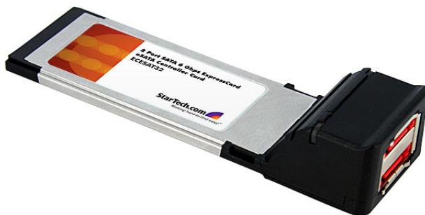
The ECESAT32 2 Port ExpressCard eSATA Controller Card (6 Gbps) offers simple connectivity between a laptop computer with ExpressCard slot and eSATA 3.0 devices - a cost-effective solution for connecting high-speed storage, such as High RPM Hard Drives and Solid State Drives (SSD), which in turn allows for easier data backups and archiving.
