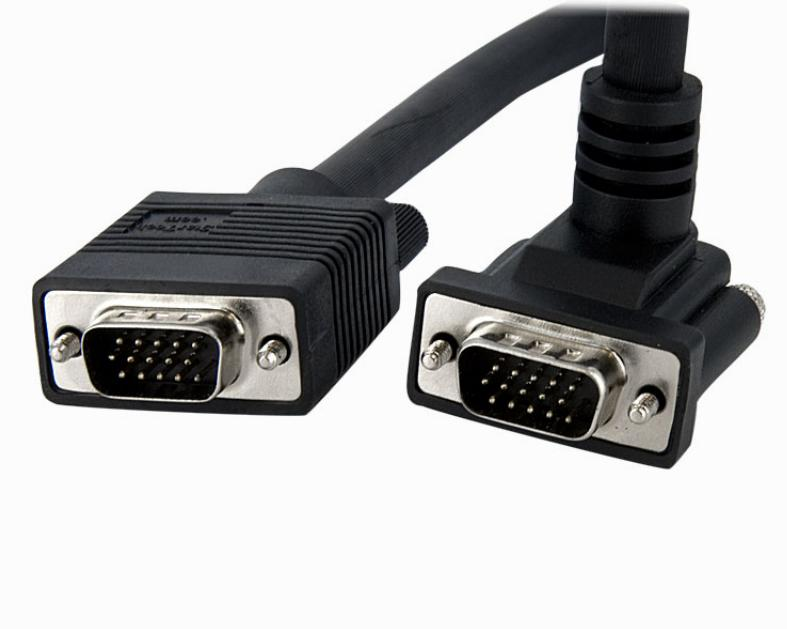
This 10ft upward-angle VGA cable is designed to support the highest resolutions and highest video quality possible through VGA while fitting perfectly in tight connection spaces. The cable features one standard VGA connector (HD15) and one VGA connector (HD15) that is situated on an upward angle relative to the shaft of the cable, requiring only 32.4mm of space at the connection point.
