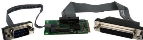
This Mini PCI Express 1S1P (PCI Express Serial/PCI Express Parallel) adapter card turns a mini PCIe slot into one RS232 (DB9) serial port and one Parallel port.
