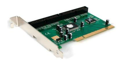
This 2 Port IDE (Ultra ATA/133) Controller Card can be installed in a PCI slot, to add more IDE storage capability to your PC.
