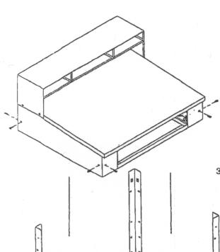
Attach four legs (4) to the desk top by attaching bolts into the two pre-welded nuts on each leg.
