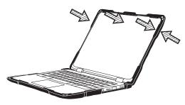
Close the case and gently press all corners together to ensure it is attached securely to the device.
