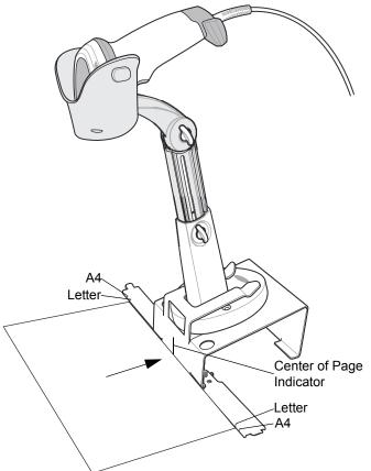
**NOTE:** Ensure to line up the edges of the paper with the marks on the document guides, if appropriate.
