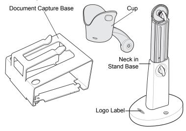
The stand can be used with the digital scanner to capture images on paper sizes up to A4 and letter (8½ in x 11 in).
