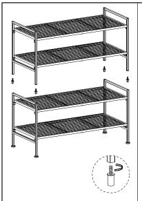
NOTE: Drawing shows 2 units stacked vertically. Do not exceed maximum height of 2 stacked units.
