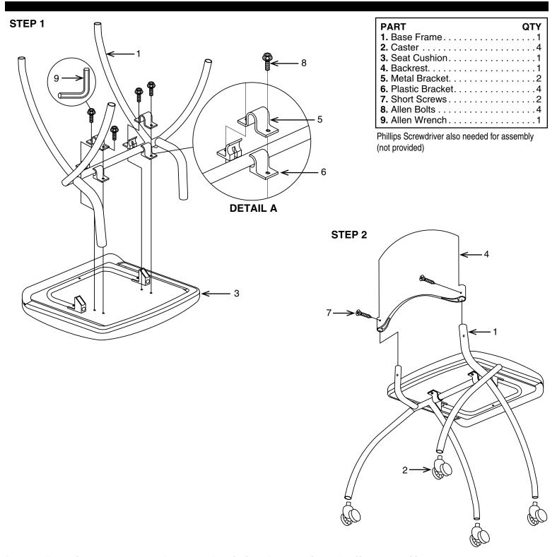
Remove all parts from carton, separate by part numbers indicated on parts list, and verify part quantities.
