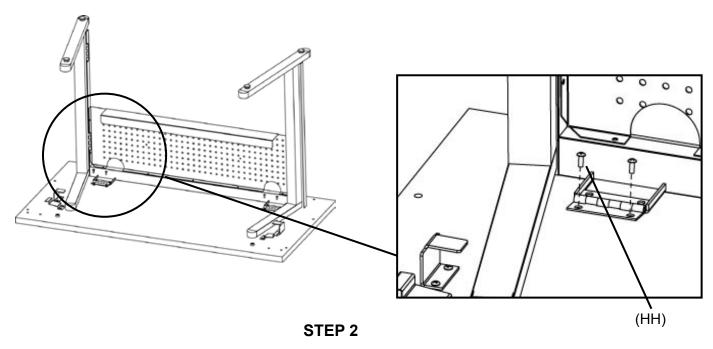
Align frame assembly with legs turned in slightly on worksurface as shown. **LOOSELY** attach with screws (HH) as shown.
