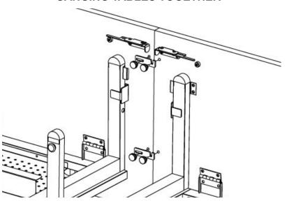
Tables can be ganged together either side to side or back to back. You can do this by attaching the ganging clips and knobs to the underside to the worksurfaces as shown.
