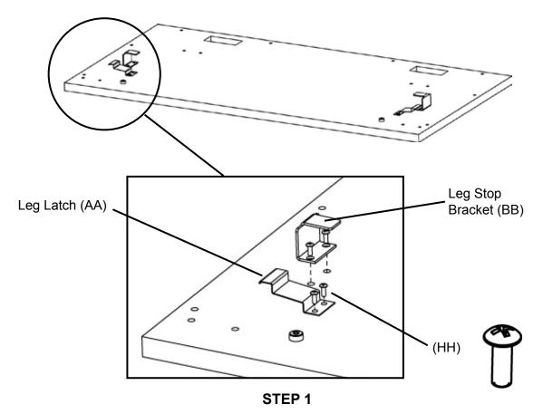
Lay worksurface down with holes facing up as shown. **LOOSELY** attach leg latches and stop brackets with screws (HH) as shown.
