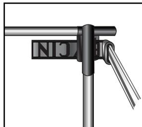
6. Last, take the Side Rail (B) and tap each end into the Black Plastic Slide Inserts (E) as shown. This completes the assembly. **Note:** Leave a small portion of the Side Rail (B) extending beyond the plastic sidepiece as shown.
