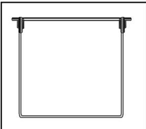
4. Lightly tap this unit onto the "U" Frame (C). Repeat steps 2-4 with another set of parts. Once complete, these assemblies will be the end components of the Hanging Folder Frame.
