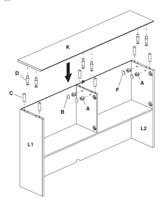
Note: For Step 3, dowels (C) are to be inserted into end panels (L1/L2) and center support (P) and not top (K).
