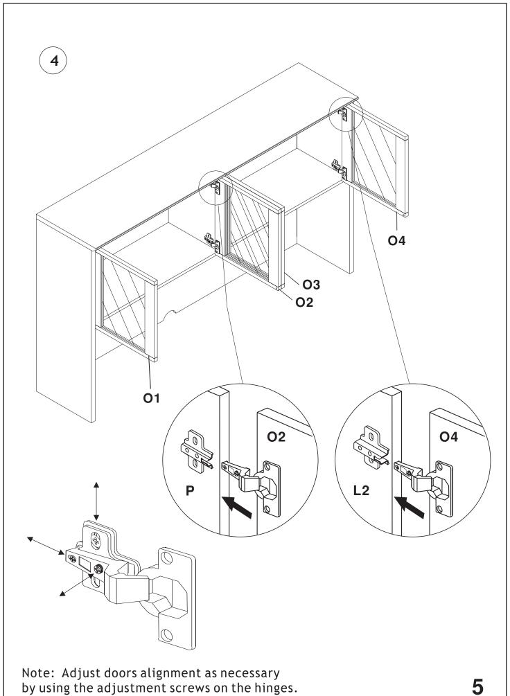
Note: Adjust doors alignment as necessary by using the adjustment screws on the hinges.
