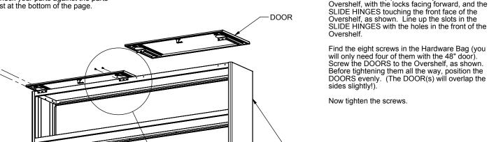
**BLACK SCREWS** Overshelf SLIDE HINGE Make sure that the slots in the SLIDE HINGE are centered on the holes in the Open Shelf. Use the slots for adjustment after both doors are on (60" and 72" only)
