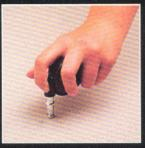
4. Tap stem firmly on hard surface or block of wood (or use hammer to tap in) until it locks into caster wheel.
